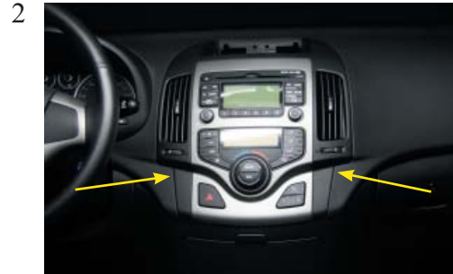
Remove the dashboard panel around the OEM radio. Use a plastic wedge.
