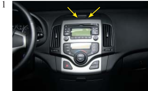
Remove the screws in the storage bin above the dashboard. At the location of the arrows.
