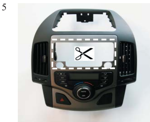
Cut out the dimensions of the new headunit out of the OEM panel.
