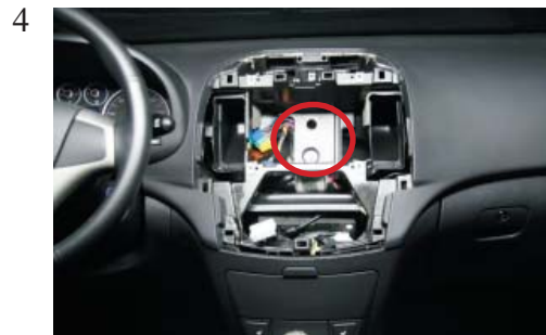
Cut off the end of the plastic frame and the metal plate that is circled(see photo).
