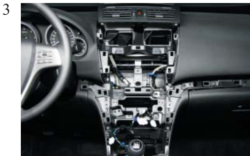
Remove the surrounding around the gear leveler. Remove the air shafts above the OEM radio.
