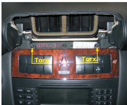
Remove ventilation shaft and remove 2x Torx 20. Then remove panel.
