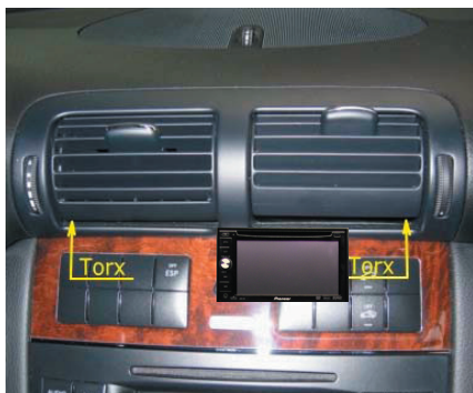
Remove 2x Torx 20 and turn ventilation shaft down, use a screwdriver to unlock the locking clip
