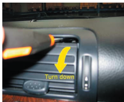
To turn ventilation shaft up, use a screwdriver to unlock the locking clip
