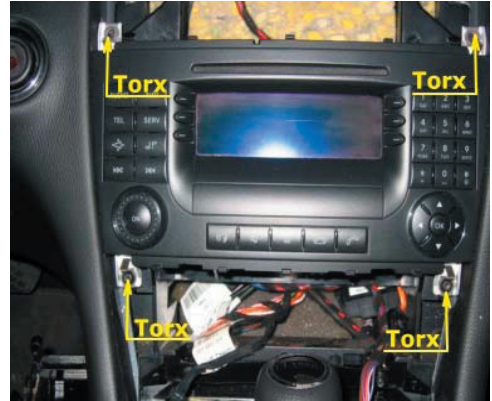
Remove 4x Torx 20 and remove original head unit
