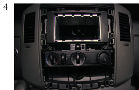
Place the replacement frame. Place the 2-Din metal bracket.
