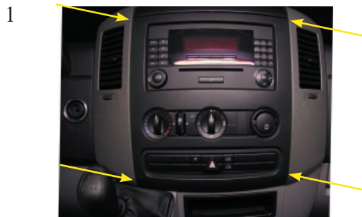
Remove the plastic panel. Use a plastic wedge.
