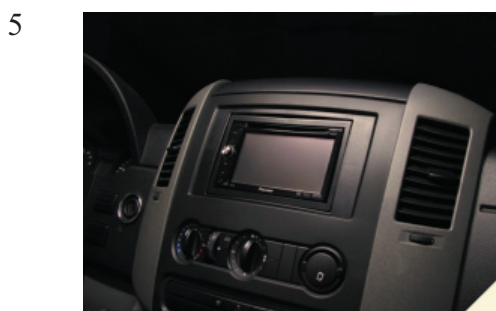
Place the headunit and the radio trim.
