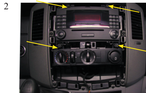
Remove the original radio. This is tighten by four screws.
