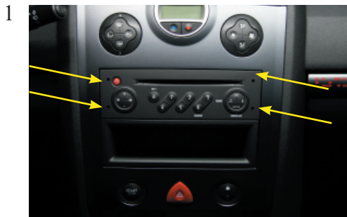
Remove the radio using the original radio release keys.
