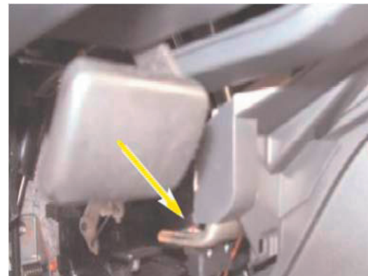
Remove locknut from head unit. At drivers side underneath the dashboard.
