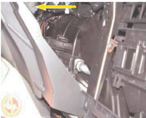
Remove locknut from head unit. At passenger side underneath the dashboard.
