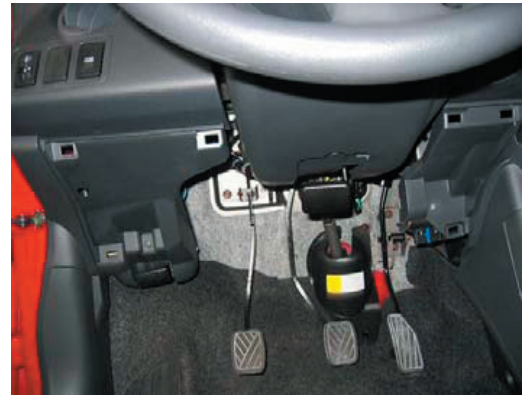
Remove dashboard cover under the steering wheel by pulling.
