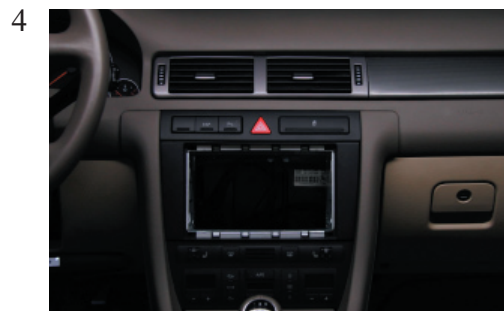
Place the 2-Din metal bracket and tighten the bracket by four screws.
