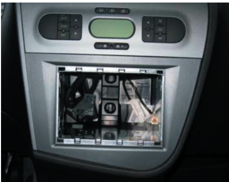
Connect all wiring and place head unit.
