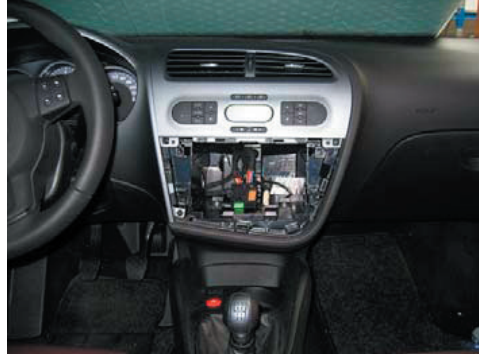
Place replacement panel for Seat Leon 05-> incl. metal bracket.
