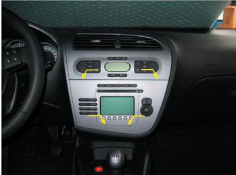
Remove original radio. Use radio removal keys at the location of the arrows.
