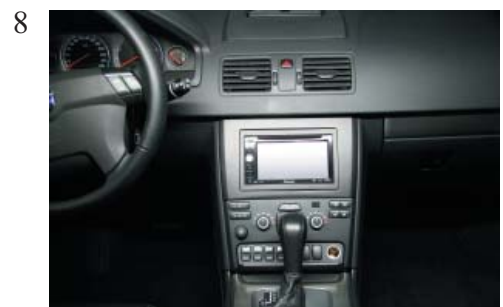
Place the new headunit and the radiotrim.
