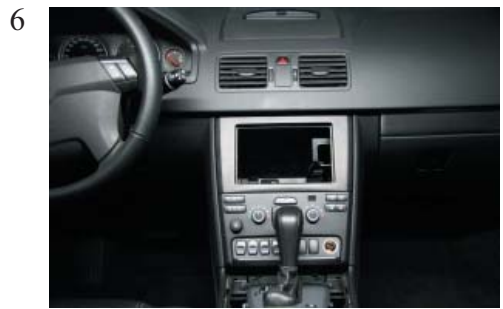
Place the oem panel with the new 2-Din panel in the dashboard
