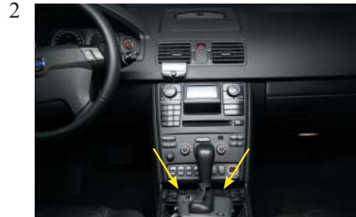
Remove the two torxs screws. Pull the original radio unit forwards.
