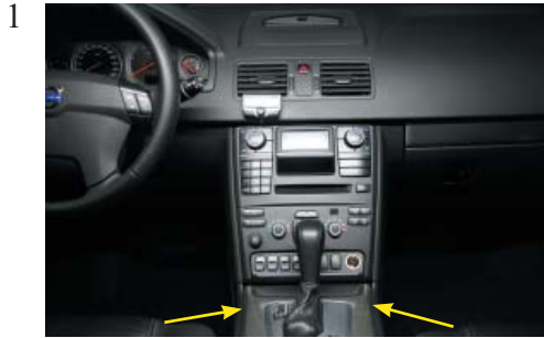
Remove the surrounding around the gear leveler.
