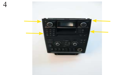
Remove the radio panel from the climate-control unit.
