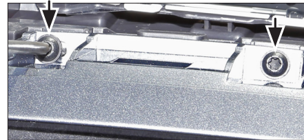
4. Remove OEM head unit by pulling it towards your direction
