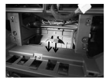
Before insert the radio pull down the internal bracket of the radio tunnel as shown in the picture.
