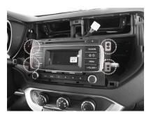
Unscrew and save the 4 screws of the original radio as shown in the picture.
