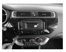
Remove the original panel, unmount the air vents; If the car is equipped with Start and Stop engine, unmount the button.
