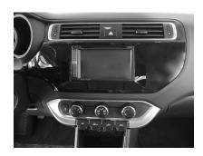
Place the clips saved before on the facia plate supplied, mount the air vents. If the car is equipped with Start and Stop engine, mount the button into the appropriate hole, otherwise install the cap with the two supplied screws. The image shows the final result.
