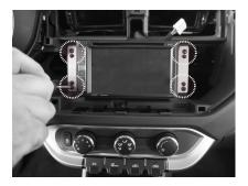
Connect all cables, verify the proper functioning of the system and insert the radio unit into the housing. Fix it with screws saved before, as shown in the picture.
