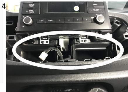
4 Remove and save the air-vents and the hazard lights button as shown in the picture.
