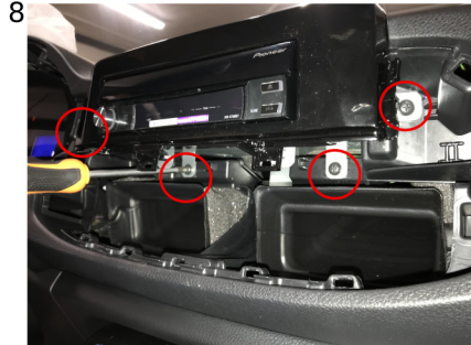
8 Connect all cables, verify the proper functioning of the system and insert the unit into the radio tunnel. Fix it with the screws saved and the bolt before as shown in the pictures.
