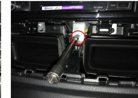
8 Connect all cables, verify the proper functioning of the system and insert the unit into the radio tunnel. Fix it with the screws saved and the bolt before as shown in the pictures.
