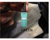
1 After the dashboard disassembly, take the two USB connectors supplied that must be connected to these two radio connectors.
