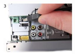
3 Connect the two USB connectors to the USB connectors of the head unit.
