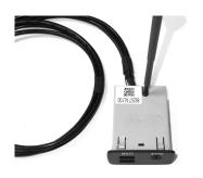
Use the screw saved before to fix the PCB to the tan cover.
