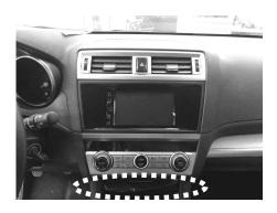
Take out the original AUX/USB, circled in the image, under the clima controls.
