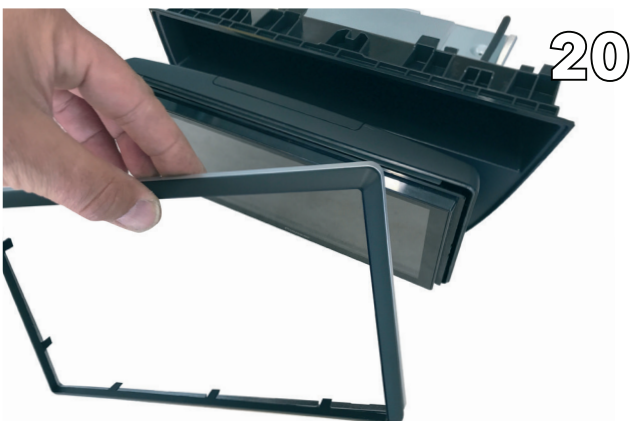
Install the front cover with the chrome bezel
