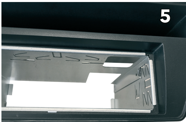
Slide the metal cage into the vehicle with the opening on top
