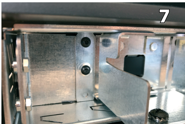
Close the locking tabs and secure with the necessary screws
