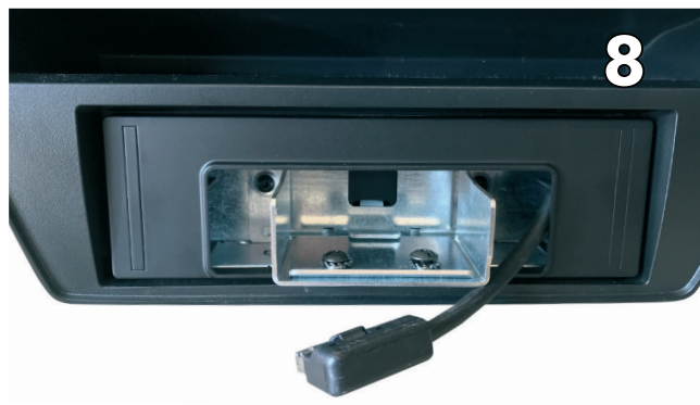
Put the DIN cover over the unit
