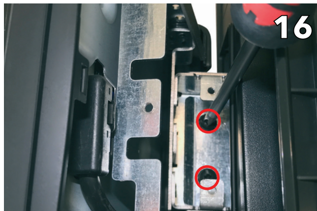
Slide the screen into the support and secure with two screws
