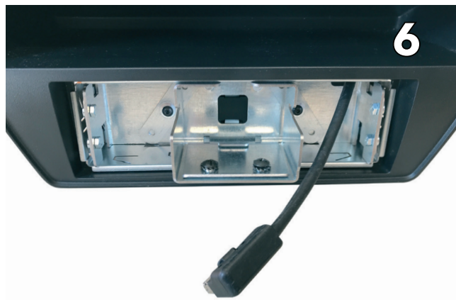
Whilst sliding the silver box in the car pull the display cable through using some tape (not included)
