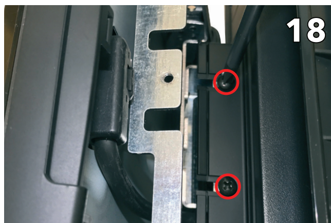
Install the neck cover onto the screen and fix the screws
