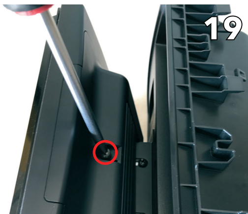
Slide the cover onto the screen and fix the screw
