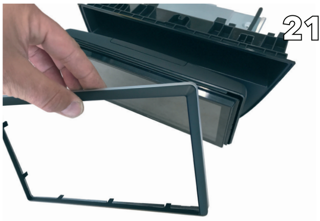
Install the front cover with the chrome bezel
