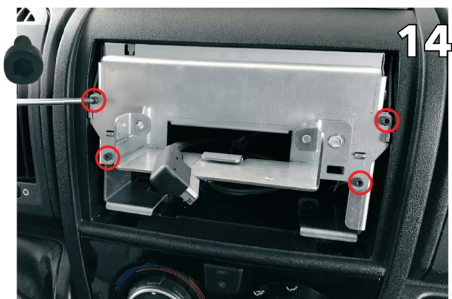
After installing the interface, slide the unit into the dashboard, routing the display cable underneath and tighten 4 small allen screws
