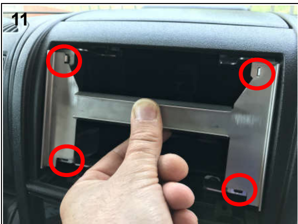
Before tightening the screws, put the installation jig in place, as shown. Insert the jig in the indicated square holes. Fix the two screws for each bracket as shown in the pictures 12A and 12B.
